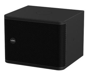
The Venu 112 V2 is a single 12" compact low frequency enclosure, providing a frequency response of 40Hz  $\pm 3$  dB and efficiency of 99dB1w/1m. Features include a tough 12" high excursion transducer with a 4" voice coil and a strong enclosure made entirely from 15 mm multi-laminate birch plywood.
